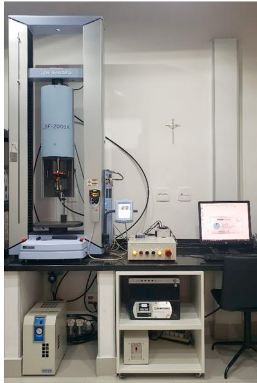
Fig. 2. Shimadzu USF-2000 ultrasonic machine at LABFADAC's laboratory.
